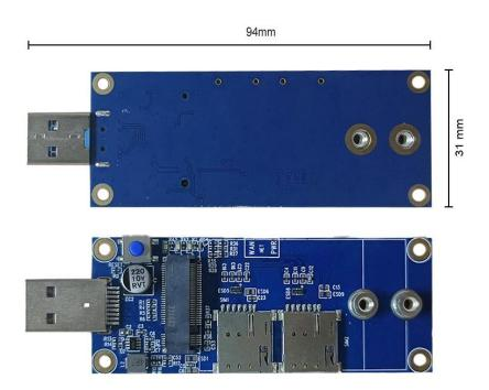
This product is suitable for 42\*30mm and 52\*30mm LTE modules with M.2 B key interface.
