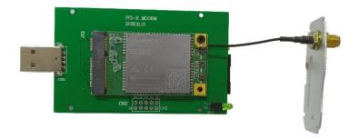
3.SIM card insertion method:uses drawer card holder. Please use card reader or pointed object to counter the small dot, pop out the card slot, and insert or remove the SIM card accordingly.
