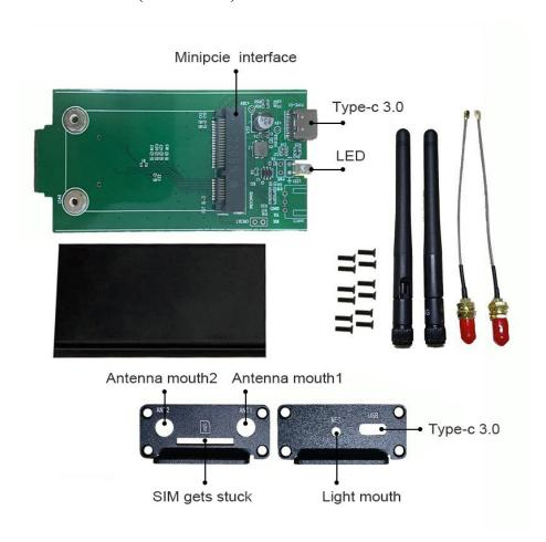
This product is suitable for 42mm\*30mm/52mm\*30mm, B key M.2 interface module.
